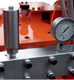
Stainless steel pump-head. Integrated cooling for plunger-seals.
