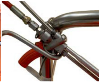
Stainless steel top-frame with gun rest / lance holder.
